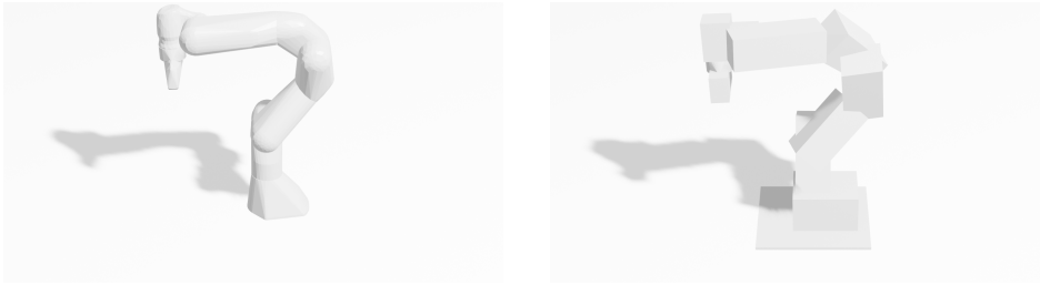
(a) : Original robot mesh. 10^4 vertices. (b) : Simplified robot mesh. 10^2 vertices.
